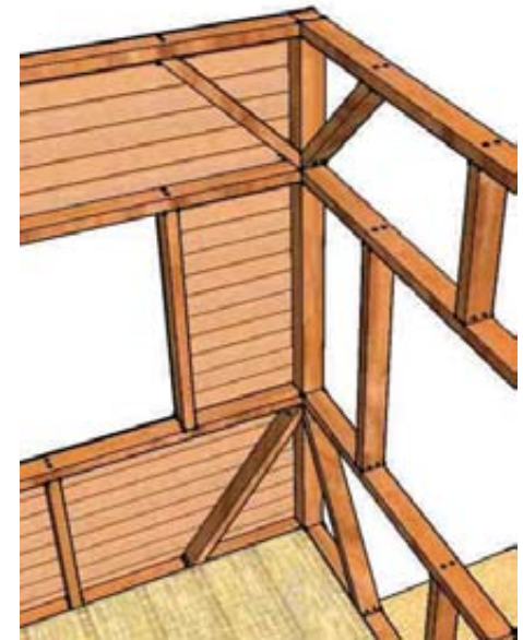
Diagonal Bracings in Timber Wall
