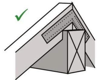
Good roofing detail with the use of a metal plate
