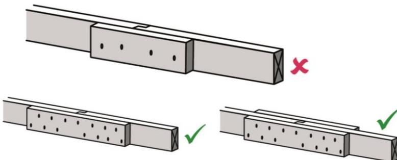
Poor joints are short and poorly nailed (above). One or two nailed plates with nails evenly distributed and at least  $\frac{3}{4}$  deep are stronger.
