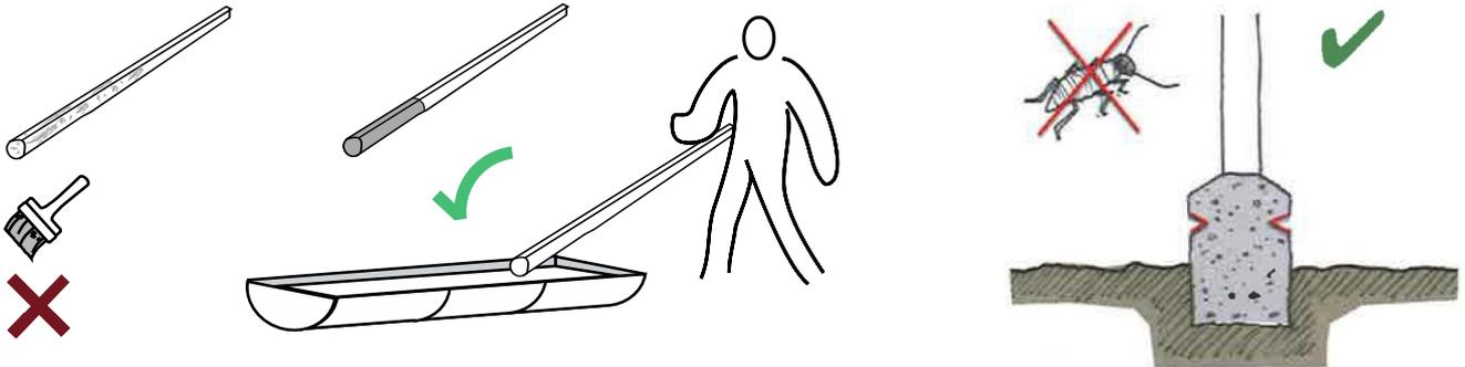
Dip the timbers in sump oil, rather than painting. Soak up to 3 ft. Prepare the dip tank from a barrel cut in half.
