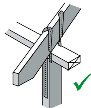
Ensure that the roof is tied down with metal straps or wires
