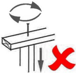
A single nail can easily twist or pull out
