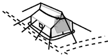
blanket or plastic sheeting covering unused door. note drainage ditches and site drainage around tent
