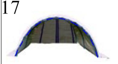
Insert end between roof sheet and poles.
