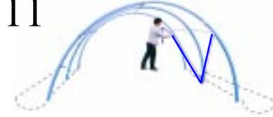
Tie rope to from first joint to centre peg to first joint at far end of shelter
