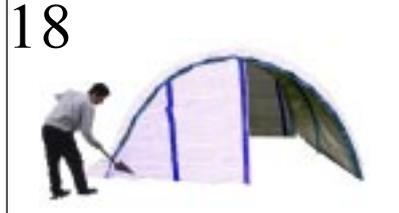
Cut remaining plastic into two to create a door. Fill trenches.
